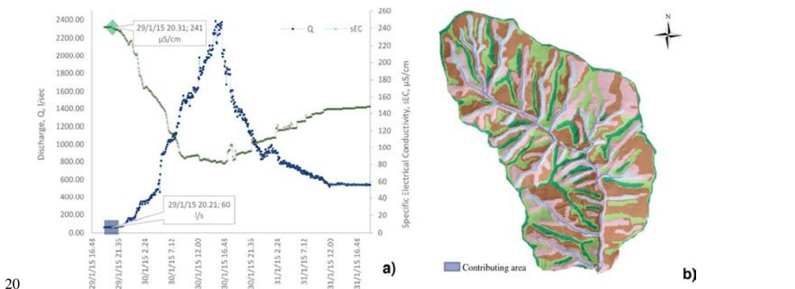
Figure 9. a) Pre-event hydro-chemograph conditions, just before the storm event, with  $Q=60$   $L/s$ , filled blue square and  $EC=240$   $\mu S/cm$ , filled green diamond, b) scenario corresponding to groundwater and decreasing groundwater ridging contribution to streamflow running exclusively along the riparian corridor and main streamflow.
