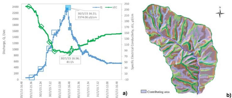
10 Figure 13. Final hydro-chemograph conditions, after approximately 100 mm of rainfall inducing a peak discharge
