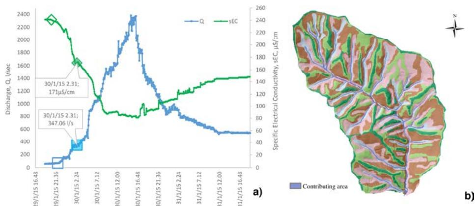
Figure 10. Initial hydro-chemograph conditions, just after the beginning of the storm event, with  $Q=350$  L/s, filled blue square and  $EC=170$   $\mu\text{S/cm}$ , filled green diamond, b) scenario corresponding to an increasing groundwater ridging and initial saturation excess contributions to streamflow. The first occurs along the riparian corridor, the second at the apical transient channels just downstream the colluvial hollows, respectively.
