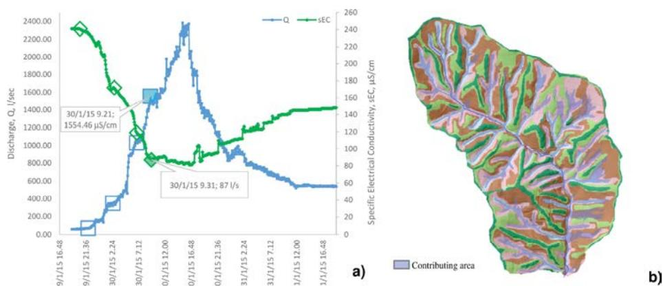
Figure 12. Advanced hydro-chemograph conditions, after approximately 80 mm of rainfall, with approximately  $Q = 1550$   $L/s$ ,
