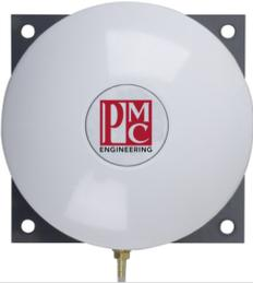
In order to reduce on-site maintenance PMC has developed the **MP 11** Moisture Protection Reference Volume. For vented gauge transmitters this provides total isolation from the atmosphere by using a custom bladder, while maintaining the high performance of the transmitter. Totally maintenance free. Please specify MP 11.
