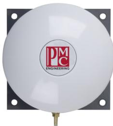
In order to reduce on site maintenance PMC has developed the MP 11 Moisture Protection Reference Volume. For vented gauge transmitters this provides a total isolation to the atmosphere by using a custom bladder while maintaining the high performance of the transmitter. This changes volume with Barometric pressure. Totally maintenance free. Please specify MP 11.
